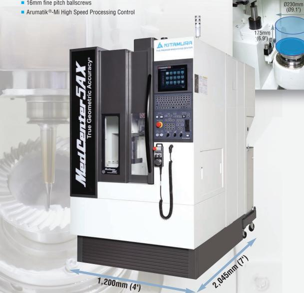
Positioning Accuracy: ±0.002mm (±0.000079") / Full Stroke Repeatability: ±0.001mm (±0.000039")
